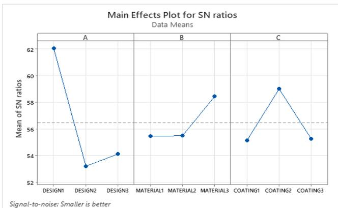
Figure 3 Main effect plot for SN ratio
